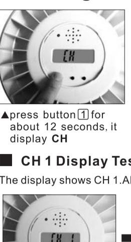
The Automatic Pill Dispenser has a built-in function to test the device. To enter the test mode, press button 1 for about 12 seconds, the CH should appear on the display. To exit test mode, press button 3.
