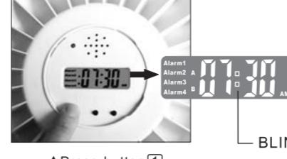
1. Press and hold button 1 for a few seconds (until the symbol ":" blinks) and then release.
