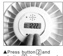
The automatic pill dispenser automatically defaults to a 24 hour time format. To switch to a 12 hour format, press buttons 2 and 3 simultaneously. The AM or PM symbol will appear on the right side of the display when the clock is in the 12 hour time format. Release the buttons when the desired time format is displayed.
