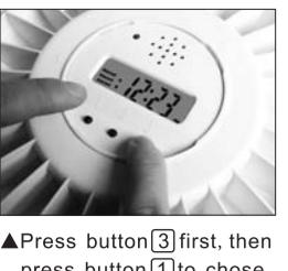
The Automatic Pill Dispenser has 3 different alarm tones and also silence to accommodate different hearing levels. Symbols A, B and A+B on the display indicate the selected alarm tone, if "silence" is selected, then neither A nor B appears on the display. To change the alarm tone, first hold down button 3 and then at the same time hold down button 1 to choose the next alarm tone. Continue to hold button 3 and press button 1 to listen to and select the different tones.
